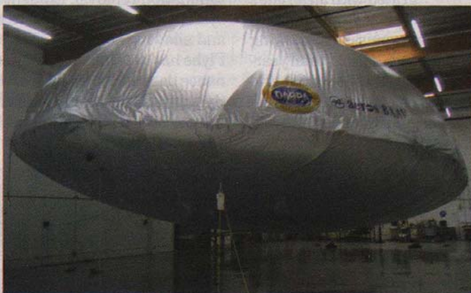
Aeros has tested a 75-ft.-long subscale version of the lightweight composite aerostructure for its planned ML866 rigid-hull hybrid airship.
